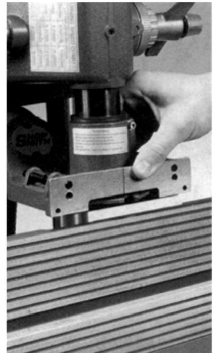
**Figure 23-16.** For surface cuts, adjust the table so it is flush with the biscuit joiner guide when fully depressed.
