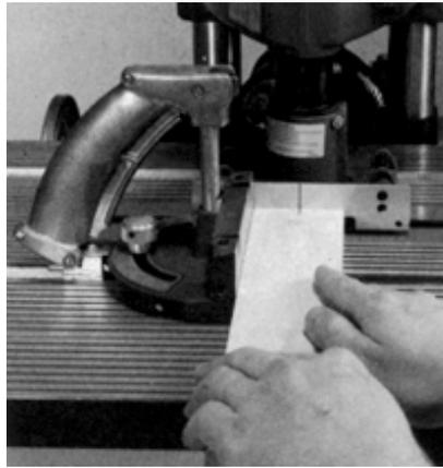
**Figure 23-13.** If the stock does not engage both pins, use your miter gauge to maintain control of the workpiece.
